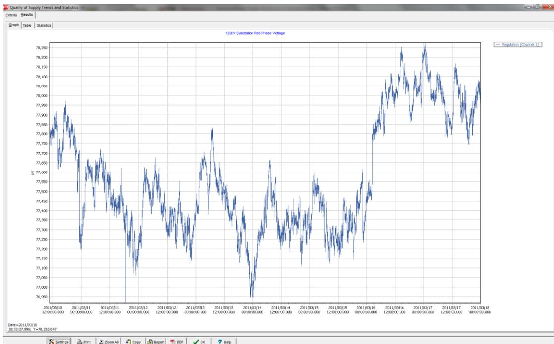
Fig. 11. 132kV substation supply voltage (10 minute mean value) variation with time.
