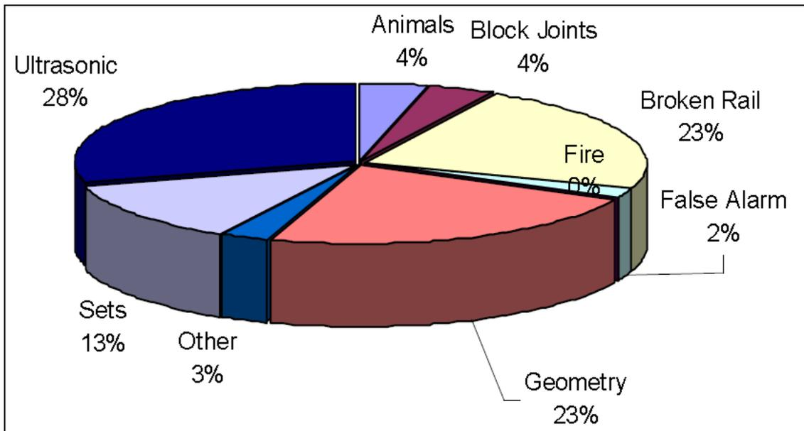
Fig. 13. Train delays due to Infrastructure.
