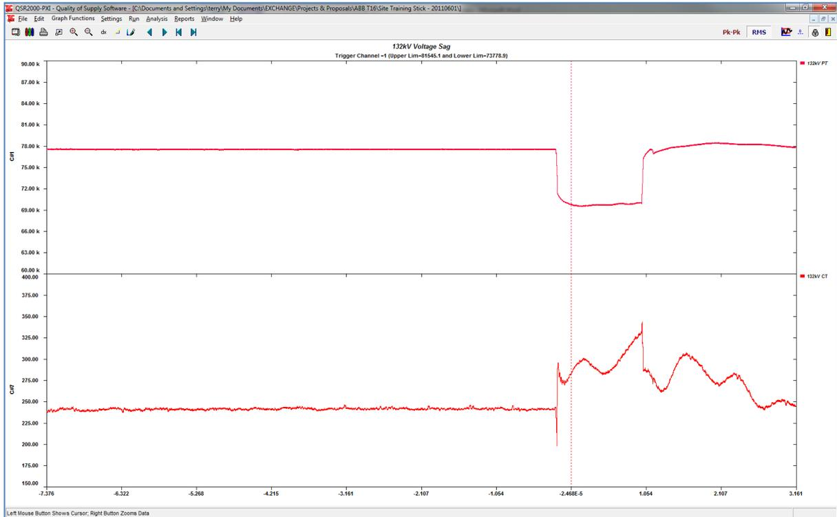
Fig. 8. Supply current (rms) to drive during a dip on 132kV substation supply.
