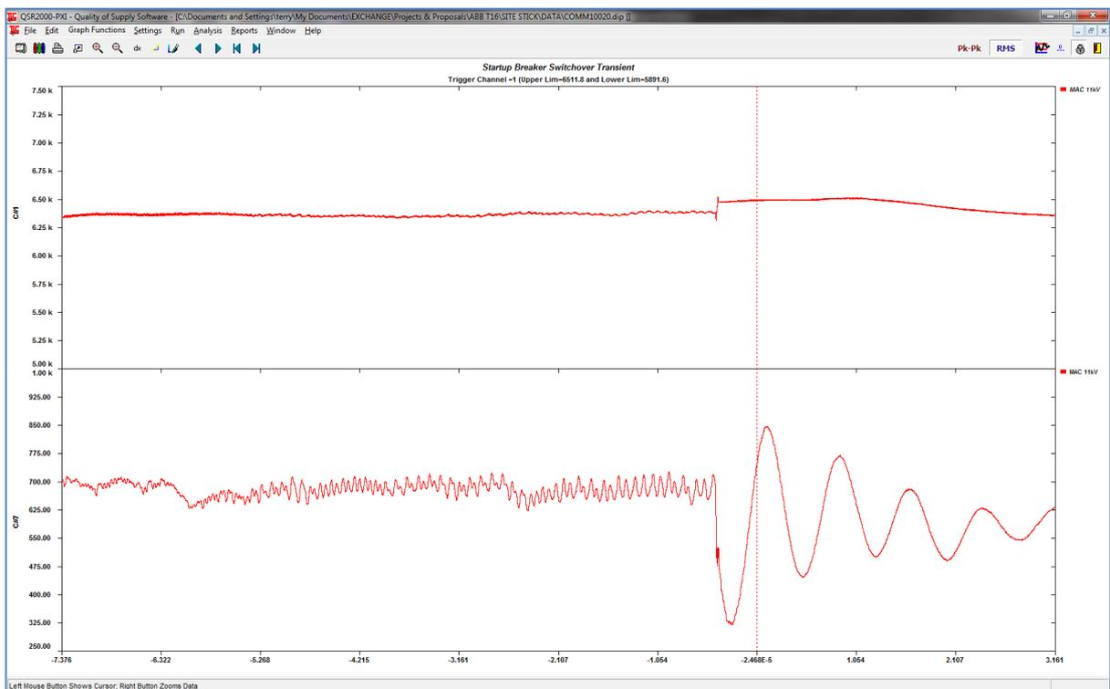
Fig. 7. Motor current waveform during LCI bypass switchover to substation supply.
