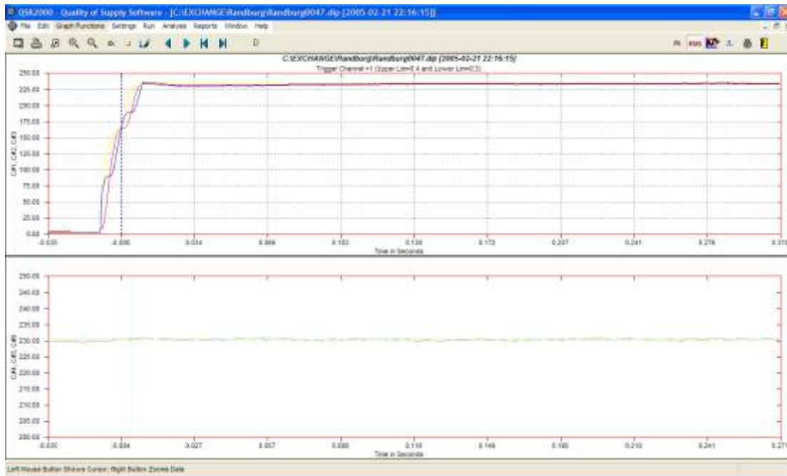
Fig 9: Incoming Supply Restored – UPS Unaffected
