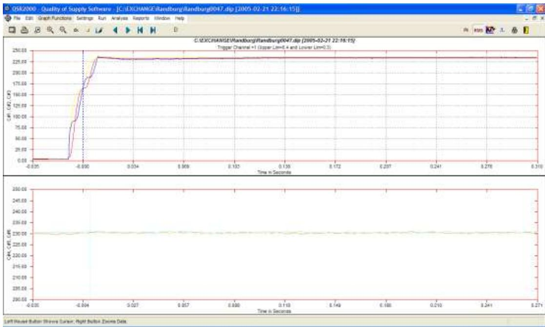
**Incoming Supply Restored with Normal UPS Output to the Load**
