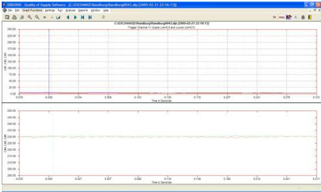
**Incoming Supply Failure with Stable UPS Output**
