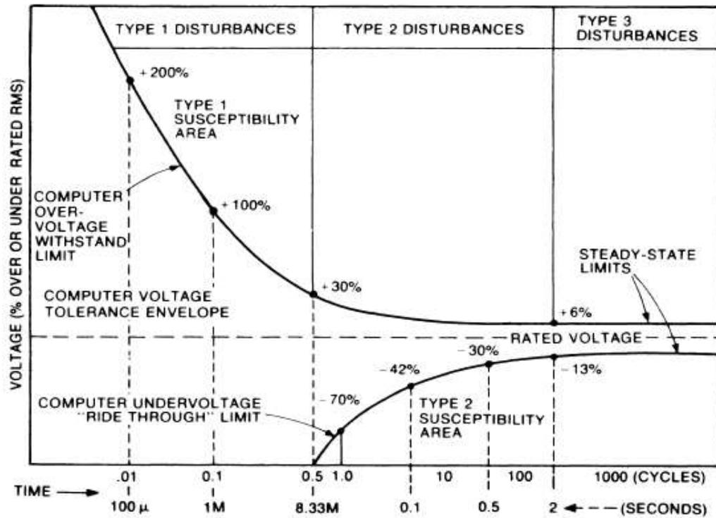
There have been a number of revisions to this curve for various industries and types of equipment. They all provide guidelines to the voltage tolerance limits within which equipment should function satisfactorily. Similar data in South Africa (NRS048-2:1996) is presented in the form of a two-dimensional plot of dip depth and duration as shown below.
