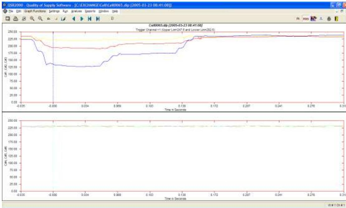
Severe Voltage Dip on the Supply has no effect on the UPS output
