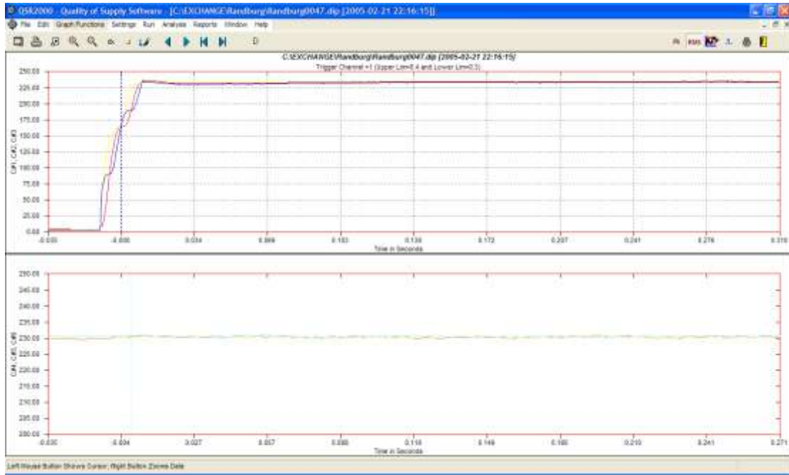
Figure 10: Incoming Supply Restored with Corresponding UPS Output
