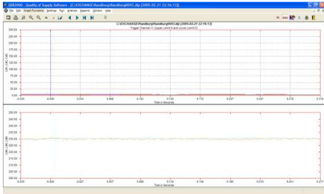
Figure 9: Incoming Supply Failure with Corresponding UPS Output
